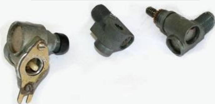
Smiths instrument angle drives, nominally 1-1 non reversing
