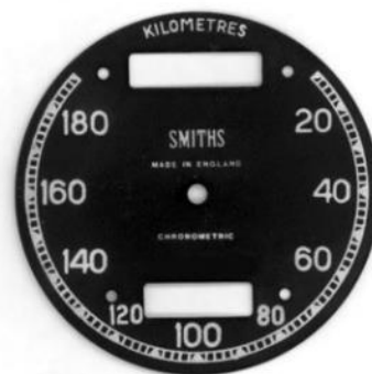
180kph chronometric speedo for metric areas. 180 km/h
